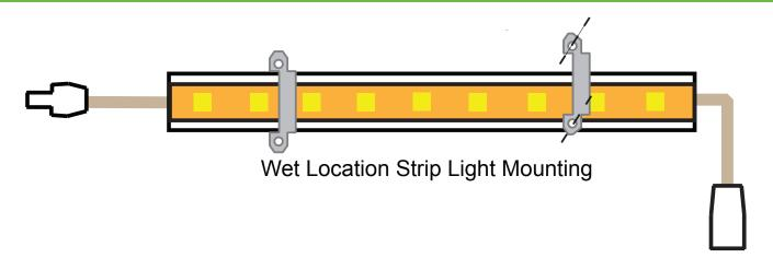
Wet Location Strip Light Mounting Clips can be used two clips per foot, but more or less may be used depending on the installation.
